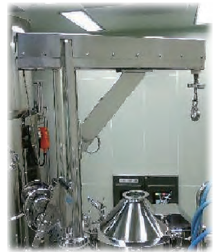
Cleanroom Jib Crane
