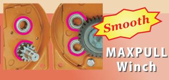
Ball bearings are used on all rotating parts such as gear and shaft.
