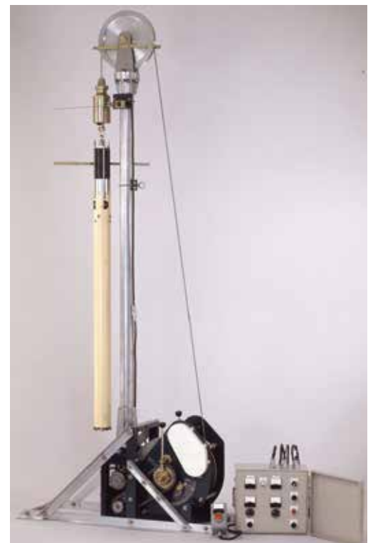
"Shallow ice coring system" for the 29th and 30th Japanese Antarctic Research Expedition
